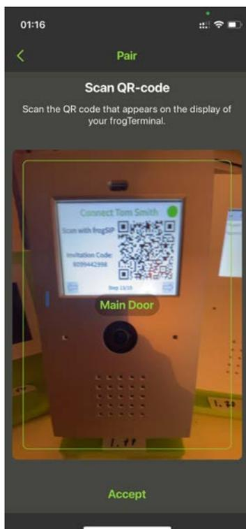
Use your smartphone camera to scan the QR code displayed on the frogTerminal device screen.
